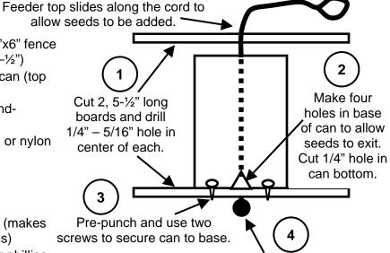
Thread cord through bottom board, tin can, and top board. Secure bottom with knot and the top with a loop to hang feeder.
